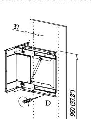
Step 3: Screw Ironing Board(F) to mechanism(A) using 6 machine screws(E).
