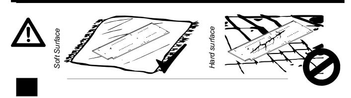
After unpacking, place the panels on a soft surface.
