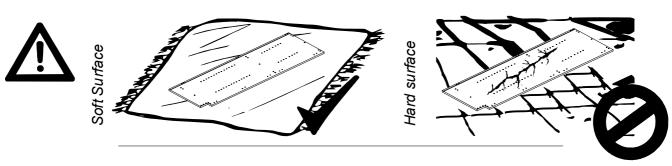
After unpacking, place the panels on a soft surface.
