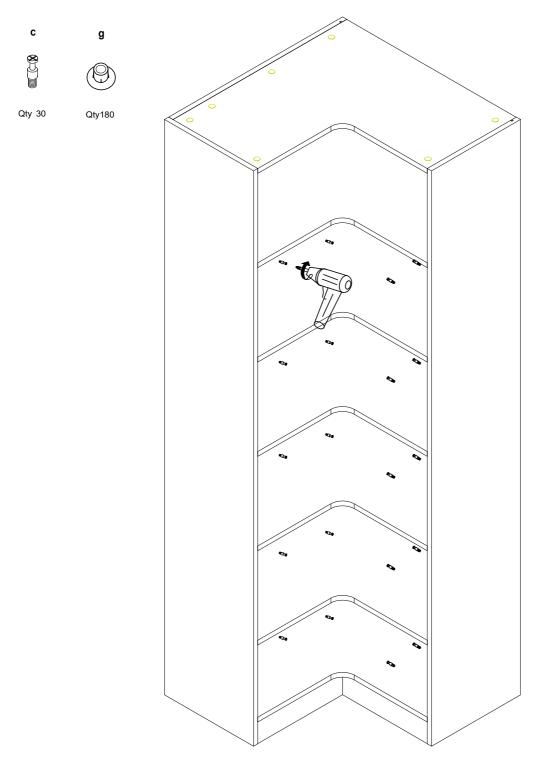
When placing two cabinets next to each other use below hardware to connect the two cabinets for extra strength
