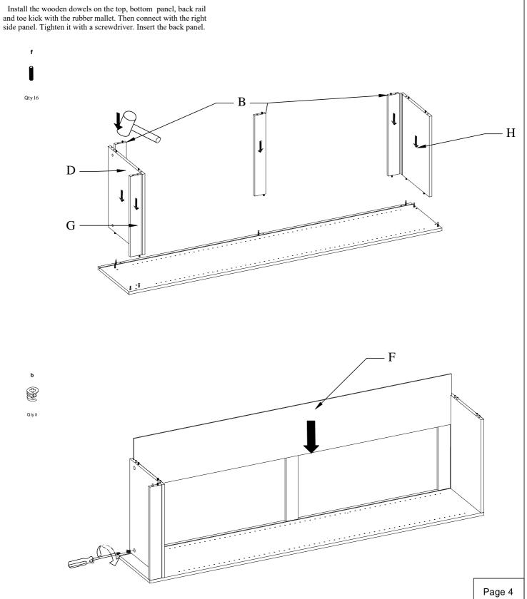
Fasten the left side panel with a screwdriver, then paste perfect paste to the hole.
