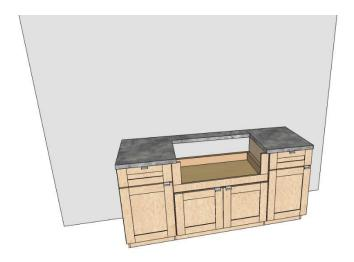
Step 2: Cut top of wall cabinet for plumbing, add support for sink, build toe base, add stiles to frame around the sink apron
