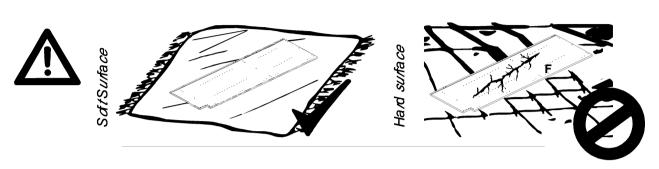
After unpacking, place the panels on a soft surface.
