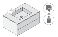
d. Seal the joint between the washbasin and the wall with anti-mould silicone. Smooth the silicone bead and let it dry for at least 24 hours.
