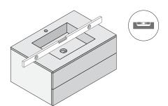
C. Clean the joint between the washbasin and the wall with a degreasing agent such as alcohol, acetone or other suitable agent. Clean the rest of the washbasin surface.
