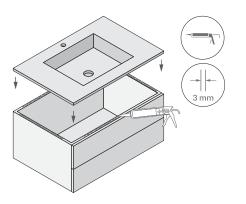
b. Immediately afterwards, place the washbasin on top of the bathroom cabinet, making sure that the washbasin is centred and levelled.
