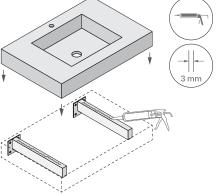
b. Immediately afterwards, place the washbasin on top of the support bars, making sure that the washbasin is centred and levelled.
