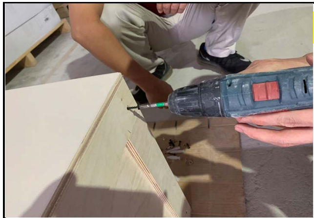
Step8(P8): After finishing inserting back panel, screwing screws through the holes at back of back panel.
