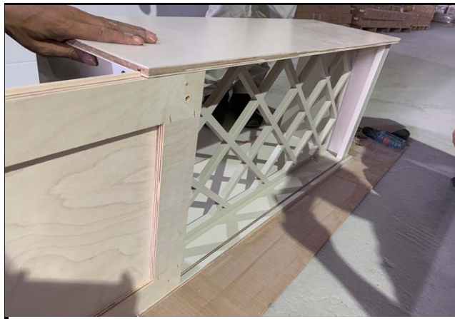
Step7(P7): After the rear grid fixed, inserting the back panel along with the back panel grooves in left and side panels.
