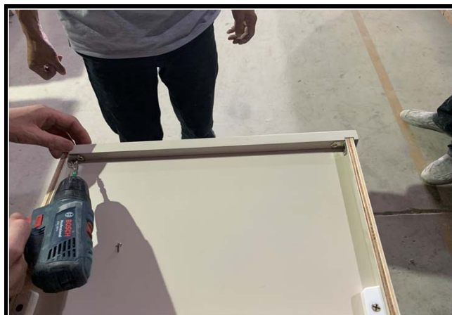
Step8(P8): After finishing inserting back panel, screwing screws through the holes at back of back panel.
