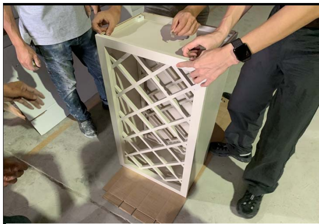
Step7(P7): After the rear grid fixed, inserting the back panel along with the back panel grooves in left and side panels.
