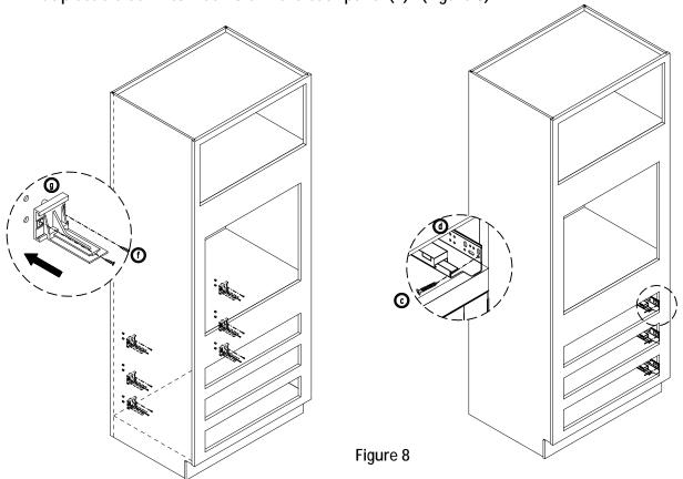
11. Assemble 3D locking device with 3 srews 6/15", to move out the slide and put drawer to click into the hook of slide with the hole in back side of drawer back . 3D locking device can just the drawer up/down, Left/Right or in/out .(Figure 9)
