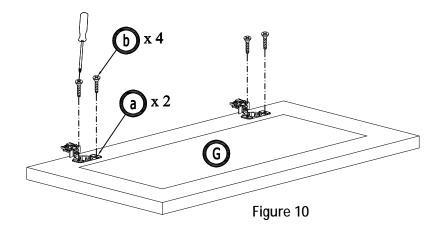
13. Assemble door with hinges to lelf and right of cabinet frame by 4 screw 4/5" (Figure 7)
