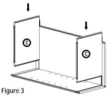
4. Installing the Remaining Panels: Insert the side panel (A) into the groove of the back panel (B) locking it into the top and bottom panels (C).
