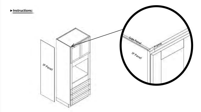
**Step 1**: Attach an IP- Island Panel or Scribe Molding to the side of the pantry or oven cabinet, keeping it flush with the face frame.
