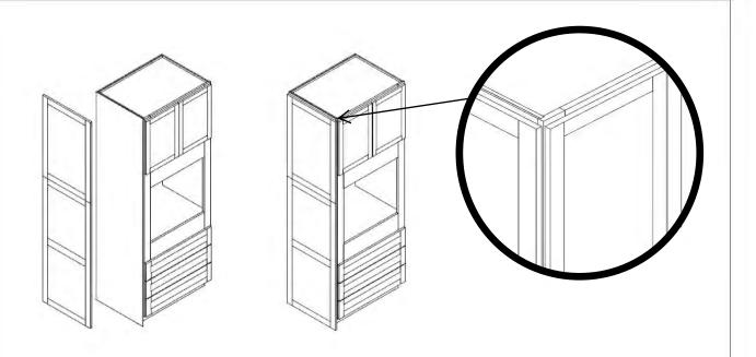
**Step 2**: Predrill pilot holes in to the side panel. Install the LDP on the side of the prepared pantry or oven cabinet. For Pantry cabinetry, position LDP panels to compliment the doors on the front of the pantry cabinet. (Recommended: 12 pcs. 1" flat head screws.)
