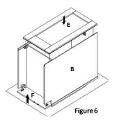
5. Install the Drawer Slide Rails: Insert the drawer side rail's back end (g) into the holder (f) previously installed (Step 4) on the back panel (E) (Figure 6). Then secure the drawer rail front end with 1/2" screws (e) using the pre-drilled holes in the face frame (A).
