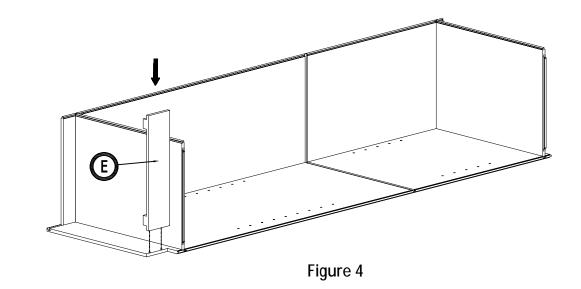
4. Install the Toe Kick : Insert the Toe Kick (E) into the free hole of side panel (A) .(Figure 4)
