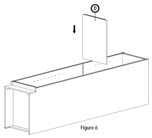
7. Install the framel: Insert the frame (F) into the groove of the side panel (A), top, bottom (C) and center panel (D). Press down until they click into place. (Figure 6)
