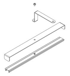
1. Assemble snuffer using screw provided.
