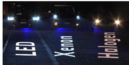
Figure 8: Different color temperatures of LED, HID/Xenon and Halogen headlights when compared side by side (exemplary)
