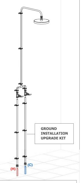
HOT & COLD INLETS INSTALLED AT GROUND LEVEL (GROUND-FED)
