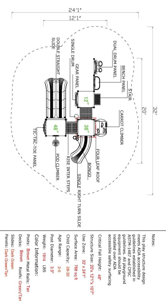
guidelines. All playground guidelines established in accessible safety surfacing equipment should be meets ADA accessibility installed over ADA ASTM-1487 and CPSC This play structure design
