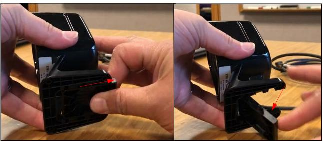
5. If installing the Riser, first open the Riser door to facilitate plugging in the cable. Pull the riser door straight out, then push down to swing open.
