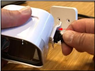
4. The Scanner can now be placed in the L bracket, facing the front or on either side.
