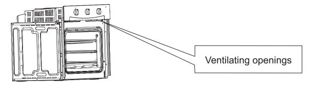
Note: the ventilating opening will coninue working for 15 minutes after the oven stops cooking.
