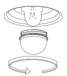
Switch off the mains power supply to replace the interior light, switch off the mains power supply and unscrew bulb. Replace with an identical bulb (230-240V~ 25W) that can withstand very high temperatures.
