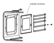
The side walls of oven are coated with self-cleaning enamel. The surface cleans itself while the oven is working. We recommend heating the oven without any food at regular intervals to complete the self-cleaning process.
