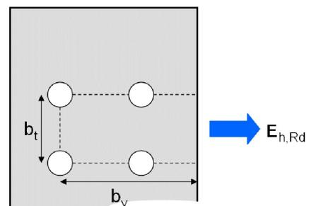
**Figure 12 Horizontal block tearing**
