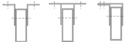
**Figure 2 Site assembled connections to mullions**
