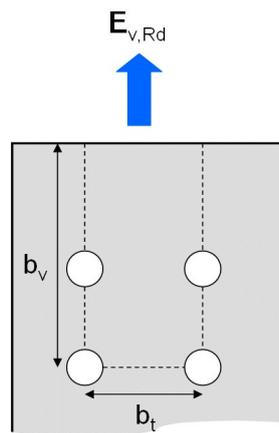
**Figure 13 Vertical block tearing**
