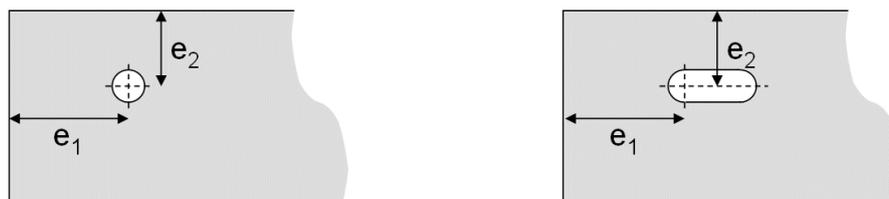
Figure 4 Edge clearance for round and slotted holes
