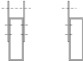
**Figure 3 Factory assembled connections to mullions**
