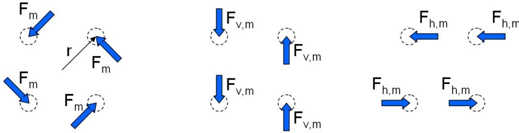
Figure 9 Forces due to applied moment
