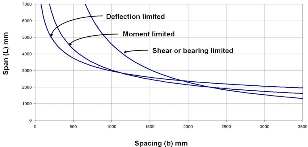
Figure 3 Limiting curves for different failure criterion
