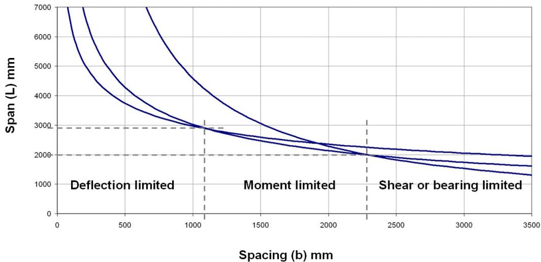
**Figure 4 Failure criteria related to different span/spacing**
