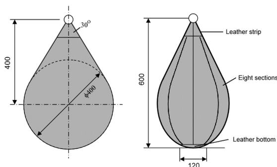
**Figure 2 Spheroconical bag**
