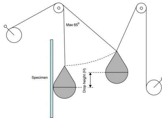
**Figure 3 Soft body test arrangement**
