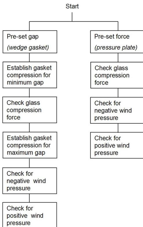
**Figure 7 Design check for glazing gaskets.**
