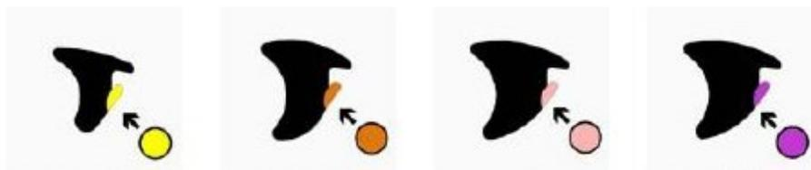
**Figure 8 Colour coded anti-stretch strips on wedge gaskets**
