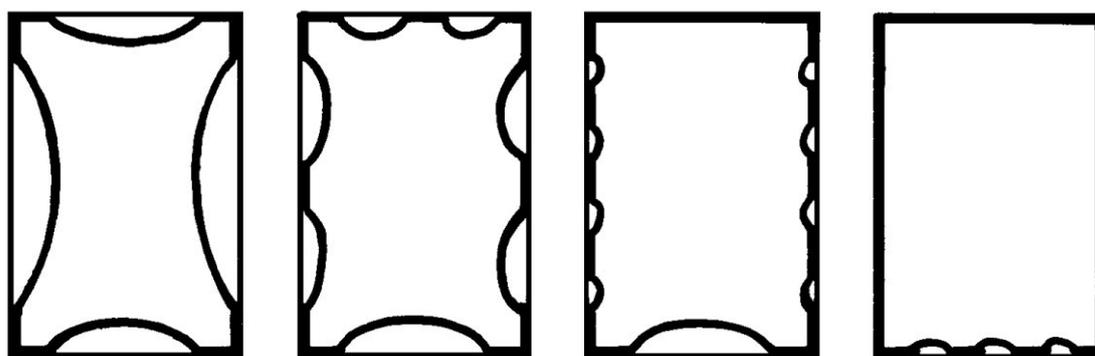
**Figure 9 Sequence for installing a picture frame gasket**
