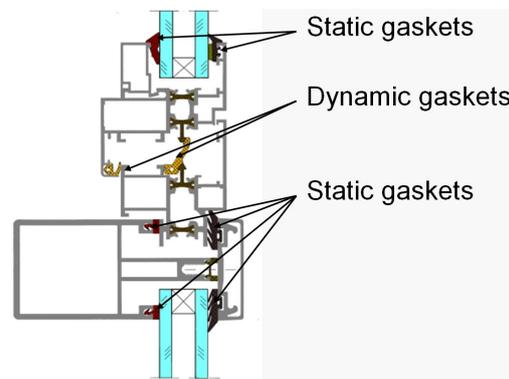
**Figure 1 Static and dynamic gaskets**
