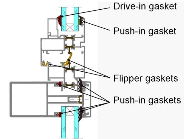
**Figure 7** Typical uses of gaskets in stick curtain wall
