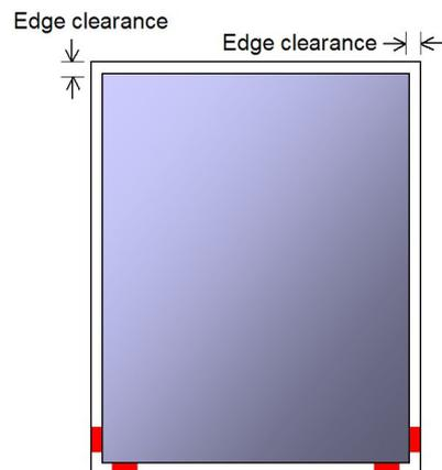
**Figure 2 Edge clearance and setting blocks**
