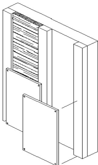
**Figure 3** Flat sheet cladding supported on timber battens
