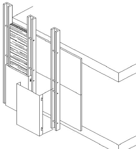
**Figure 4** Metal cladding panels used as a rainscreen supported on rails spanning between floors
