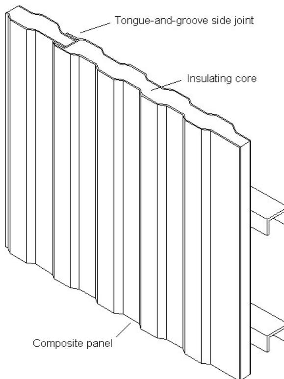
**Figure 2** Composite panel with tongue and groove joint
