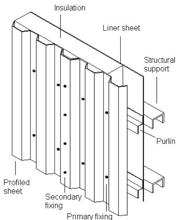
**Figure 1** Site-assembled profiled sheet metal system
