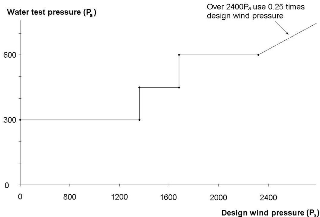
**Figure 2** Watertightness test pressure appropriate for different levels of peak wind pressure
