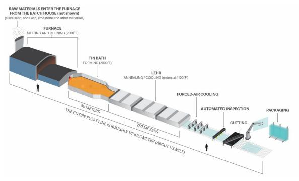
Figure 7 – Schematic of process for uncoated flat glass production (Images provided by Guardian® Glass)
