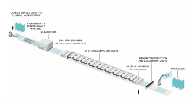
Figure 8 – Schematic of process for coated flat glass (Images provided by Guardian® Glass)
