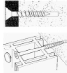
Figure 8.12 Self drilling masonry fixings
