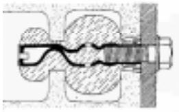
Figure 8.11 Resin fixing with net sleeve
