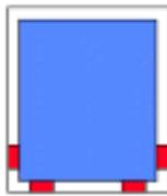
Figure 7.11 Setting and location blocks (curtain wall)
