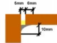
Figure 5.7 Fillet joint minimum dimensions
