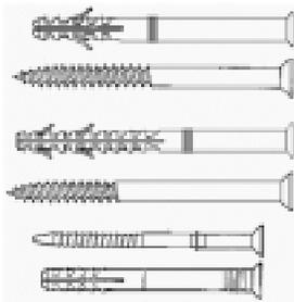
Figure 8.10 Frame fixings
