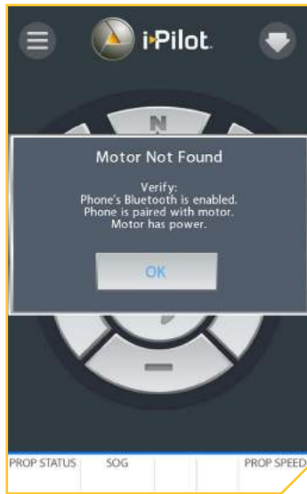
The "Motor Not Found" screen will appear when the app launches and the motor is either not powered up, connected with Bluetooth or paired to the device.
