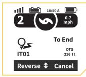
Navigating an iTrack when the boat is on course to go to the end of the iTrack.
