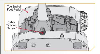
8 k. Reconfirm that the Steering Cables are tight and then carefully thread the Steering Motor Connection Wire through the top of the Wrap Drum Cover. The male plug comes from the Cable Anchor through the opening at the bottom of the Wrap Drum Cover. The wire with the female plug that runs out the top of the Cable Gear should also be pulled through the opening at the bottom of the Wrap Drum Cover.
