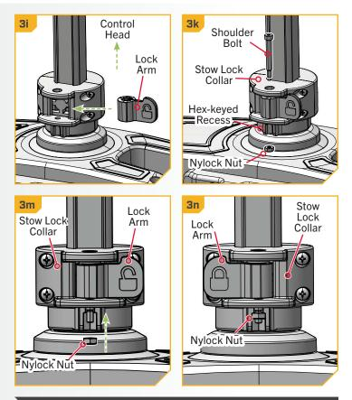
**NOTICE:** If the Stow Lock Collar is too tight, the Shaft will not move freely even when the Stow Lock Collar is unlocked. If the Stow Lock Collar is too loose, it will not securely hold the Shaft when locked.
