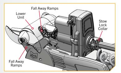
**NOTICE:** To secure the motor in place and prevent accidental deployment when stowed, lock the Stow Lock Collar  $(\square)$ . Be sure to press the Lock Arm so that it is fully seated against the Stow Lock Collar.
