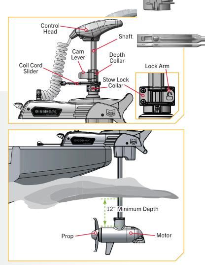
**NOTICE:** Ensure that the top of the lower unit is submerged at least 12" below the surface of the water to avoid churning or agitation of surface water.
