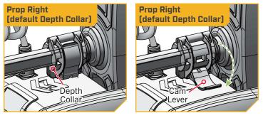
If the Stow Orientation is changed to Prop Right, the Depth Collar must be rotated on the shaft to improve accessibility. The Depth Collar is positioned correctly on the Shaft when the Cam Lever opens upward when the motor is stowed.
