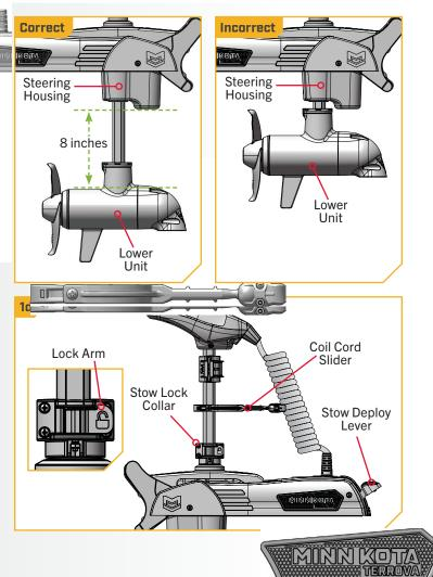
While holding down the Stow Deploy Lever, pull the e. Shaft upward to raise the Lower Unit. Tilt the Shaft into a horizontal position while guiding the motor toward the Fall Away Ramps. Pull the Lower Unit fully onto the Ramps. The Fall Away Ramps will latch upright and the STOWED O LED on the Indicator Panel will illuminate orange when the motor is properly stowed.
