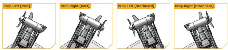
A Prop Right orientation turns the lower unit and shaft when stowed, causing the Depth Collar to open downward. This reduces its range of motion and creates an obstruction when placing the Depth Collar for a secure stow.
