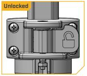
Lock Collar is locked and the Shaft is secure; when the Unlock Picon is visible, the Stow Lock Collar is unlocked and will not hold the Shaft in place. When locking or unlocking, be sure to press the Lock Arm so that it is fully seated against the Stow Lock Collar.
