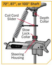
Collar is unlocked to allow the Shaft to move freely when stowing and deploying. After stowing the motor, the Stow Lock Collar is locked to ensure a secure stow. The Stow Lock Collar can also be locked to hold the motor at the proper depth when deployed in shallow water.
