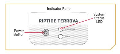
the Power button. When the Motor is powered off, the System Status LED will not be illuminated.
