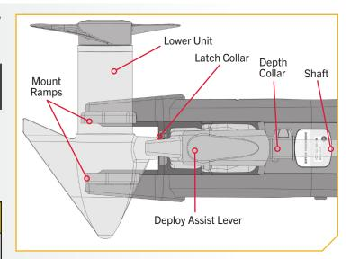
**NOTICE:** Slide the Depth Collar down and secure it against the top of the Steering Housing when stowed to secure the motor in place and prevent accidental deployment.
