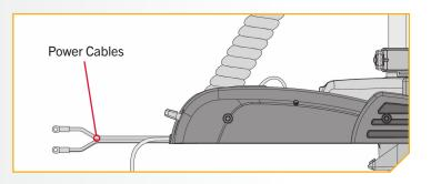
**NOTICE:** The Riptide PowerDrive has no power switch. When the Power Cables are connected to a battery, the Riptide PowerDrive is "on". When the Power Cables are disconnected from the battery, the Riptide PowerDrive is "off". If the Power Cables are connected to a breaker, the Riptide PowerDrive is "on" when the breaker is "on" and "off" when the breaker is "off".
