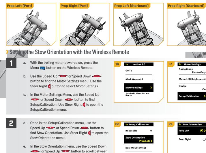
Prop Left and Prop Right. Use the Steer Right 2 button to select the desired stow orientation.
