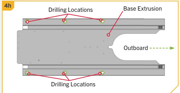
**NOTICE:** New mounting holes are required when upgrading from an Ulterra to a Riptide Instinct QUEST. New mounting holes will accommodate the higher thrust motor and ensure the installation is secure.
