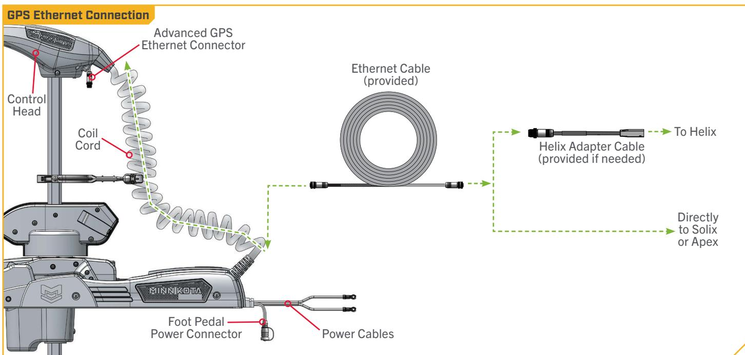
**NOTICE:** Minn Kota recommends routing the Ethernet Cable or Ethernet Extension Cable through the Coil Cord when making the Ethernet connection. The cable will be installed from the Mount to the Control Head through the Coil Cord. Bypassing the Coil Cord when routing the Ethernet Cable or Ethernet Extension Cable is not recommended.
