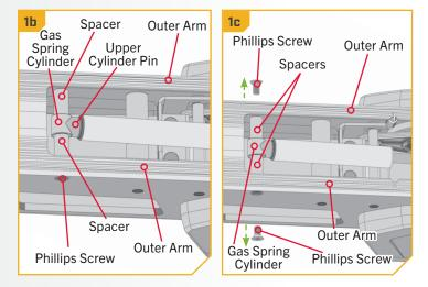
**NOTICE:** Use a #3 Philips screwdriver to remove the screws. They have a pre-applied thread locker. Failure to use the recommended tool can cause damage and prevent the screws from being removed.
