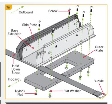
**NOTICE:** To prevent seizing of the stainless steel hardware, do not use high-speed installation tools. Highspeed installation tools will cause the hardware to gall and make disassembly challenging.
