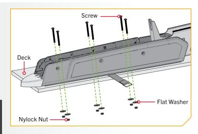
**NOTICE:** To prevent seizing of the stainless steel hardware, do not use high-speed installation tools. Highspeed installation tools will cause the hardware to gall and make disassembly challenging.
