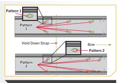
**NOTICE:** If Pattern 2 is used, the Hold Down Strap must be removed to access the mounting holes in the base of the Mount. Use a #2 Screwdriver to remove the side plate.
