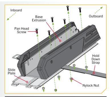
**NOTICE:** To prevent seizing of the stainless steel hardware, do not use high-speed installation tools. Highspeed installation tools will cause the hardware to gall and make disassembly challenging.
