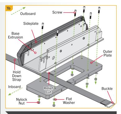
**NOTICE:** Depending on the bolt pattern used to install the Ultrex Mount to the Outer Plate of the Quick Release Bracket, the Right Sideplate may need to be removed to access the mounting holes in the base of the Mount. Use a #2 Screwdriver to remove the Right Sideplate if necessary.
