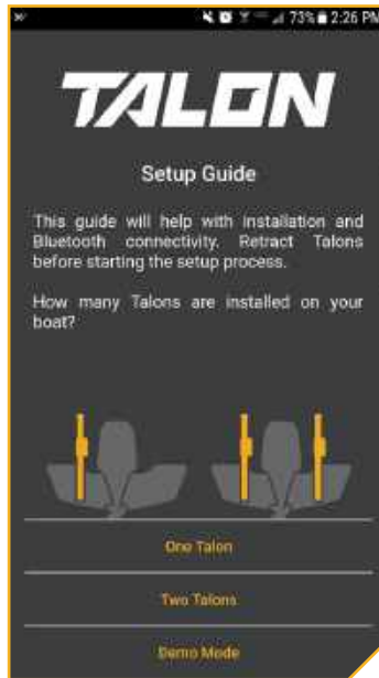
The Setup Guide appears after the Disclaimer when the device is not paired or actively communicating with a Talon.
