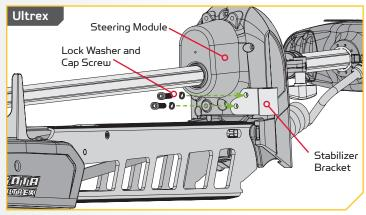
**NOTE:** The two 5/16-18 Nylock Nuts (Item #12) are not used when installing on the Ultrex.
