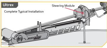
NOTE: The MKA-50 Stabilizer Kit can be installed on the left or right side of the Bowguard/Steering Module. When mounting the kit onto the Ultrex, the two Nylock Nuts (Item #12) are discarded because the bolts are secured directly into the Steering Module. The two Lock Washers (Item #16) are not used when installing on the Fortrex.
