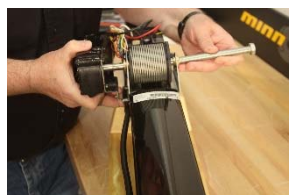
Figure 13: Slide motor out and replace with 1/2" bolt
