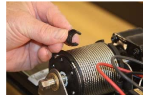
Figure 8: Spacer Clip Removed
