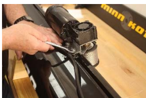
Figure 12: Remove nuts that hold the motor in place
