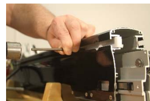
Figure 30: Use transfer punch to mark hole locations
