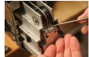
Figure 18: Retrieve rivet shanks
