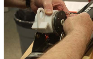
Figure 26: Remove cable closest to motor
