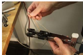
Figure 38: Route cable around tensioner
