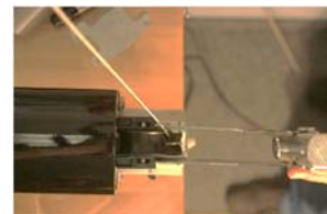
Figure 39: Installation tool arms outside of second stage
