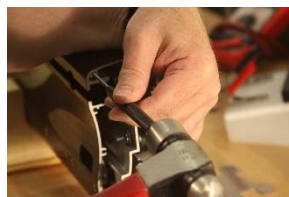
Figure 21: Drive the shanks into the body of the Talon
