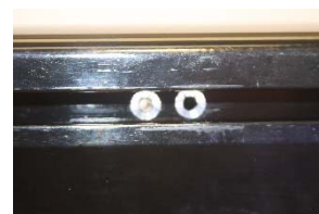
Figure 52: Tensioner aligned. Light passes through top hole.
