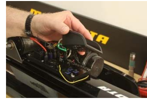
Figure 5: Carefully remove control Bezel
