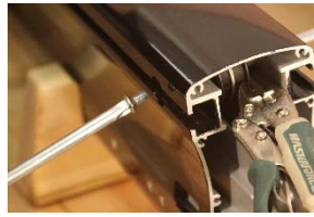
Figure 24: Use #3 Phillips drivers to remove a screw
