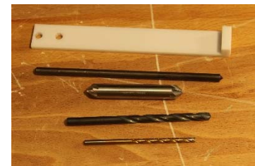
Figure 27: Tools for extrusion modification
