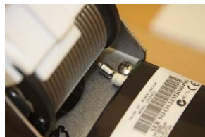
Figure 41: Cable end between above wrap drum bracket
