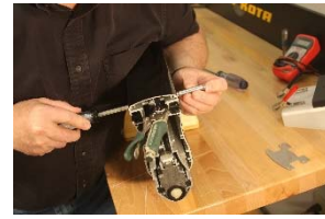
Figure 25: Push pin out then relieve cable tension
