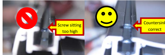
Figure 35: Top of Flat head screw from the cable tensioner kit should sit flush with lower surface of track
