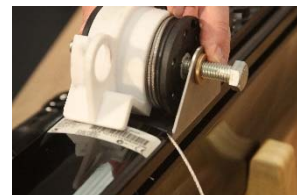
Figure 42: Cable tucked against wrap drum bracket
