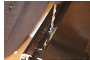
Figure 33: Complete hole with 13/64" drill bit
