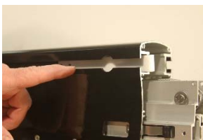
Figure 28: Position the template in the track
