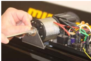
Figure 6: Remove the external e-ring
