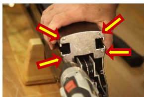
Figure 20: Remove the four rivet heads
