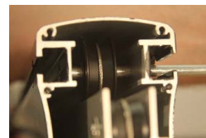
Figure 22: Water guard removed, ready for next step
