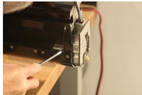
Figure 15: Pry out 3 rd stage
