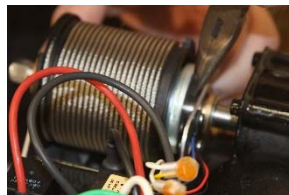
Figure 10: Retrieve the Drive Pin with pliers
