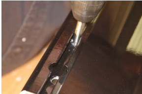
Figure 34: Countersink the holes
