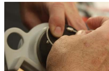
Figure 43: Insert cable end in wrap drum pocket
