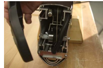
Figure 48: Top view cables properly routed
