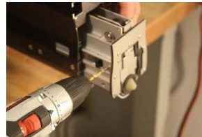
Figure 17: Drill off rivet heads
