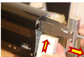
Figure 50: Pull back on the installation tool, insert block
