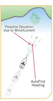
**NOTICE:** After steering to a new direction, there is a short delay before the direction is locked in to allow the compass to stabilize. When broad speed changes are made, the AutoPilot heading may change slightly. This is normal.
