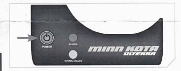
k. When the trim housing is "Learned", push and hold the power button until the motor turns off (about 3 seconds).
