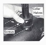
h. At this point the trim housing should be properly located with a short section of belt out the top of the housing and the lower belt block should be fully installed. There should be a significant amount of slack between the bottom of the steering housing and the lower belt clamp collar as shown.
