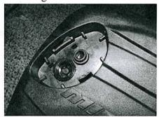
2. Remove the reed switch clip that holds the reed switch using a small flat blade screw driver.
