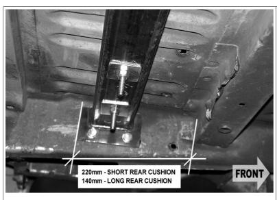
Measure from the back face of the 'spare wheel hanger' cross member (NB. The hanger has been removed from this van).
