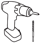
Drill with 6mm drill bit
