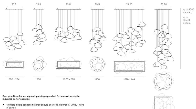
All dimensions are in millimeters (mm)
