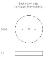
All dimensions are in millimeters (mm) unless otherwise specified.
