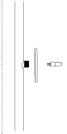
Thread the pendant mounting plate onto the stem.
