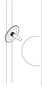
Gently thread pendant onto the stem. Be sure to carefully place the pendant so as not to damage the lamp during installation.
