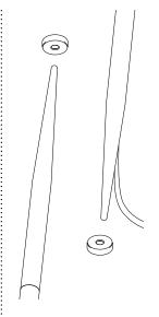
Push this end into the stem holder. The spike must rest inside the indentation.
