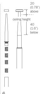
The end opposite to the cord has a spring loaded spike.
