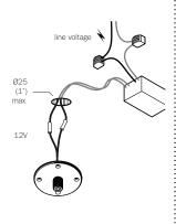
Connect power supply to line voltage.
